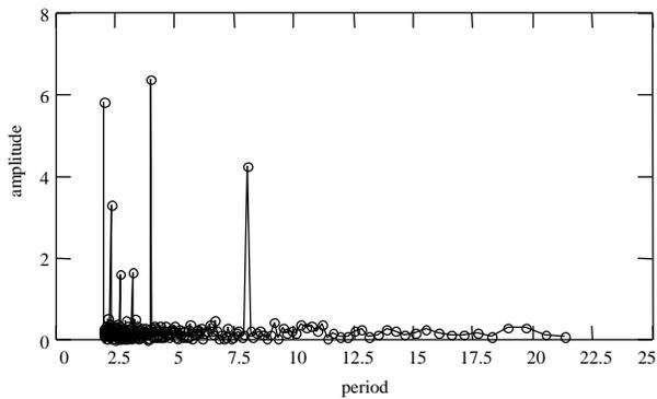
Figure 3a. Fourier amplitudes vs period of the data in Figure 2a, without the sliding scale. A period of 8 corresponds to the clock frequency, 250 MHz.
