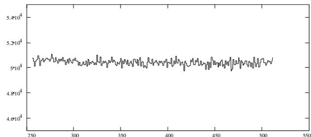
Figure 2b. The random time spectrum with the sliding scale. Note the suppressed zero on the vertical axis. The measured rms deviation is 0.46%. The expected rms deviation is 0.44% ( $\sqrt{n/n}$ ).
