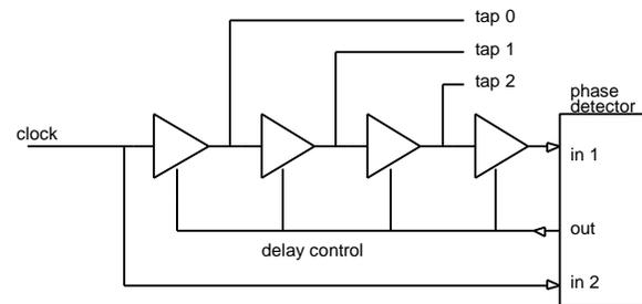
Figure 1. Tapped delay line interpolator and delay locked loop. This is used in the MTD133b to interpolate the 250 MHz clock by eight, producing an effective clock rate of 2 GHz.
