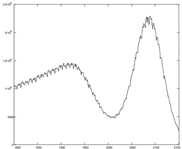
Figure 4a. Part of a Na<sup>22</sup> spectrum, without the sliding scale.
