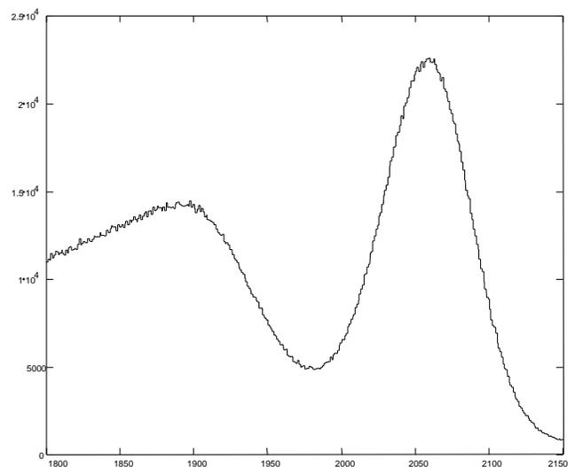
Figure 4b. The same part of a Na<sup>22</sup> spectrum, with the sliding scale. The repetitive DNL produced by the interpolator is completely eliminated.
