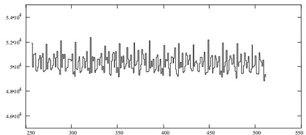
Figure 2a. The raw random time spectrum, without the sliding scale. Note the suppressed zero on the vertical axis. The peak to peak deviation is 7%, and displays the repetitive DNL of the interpolator.
